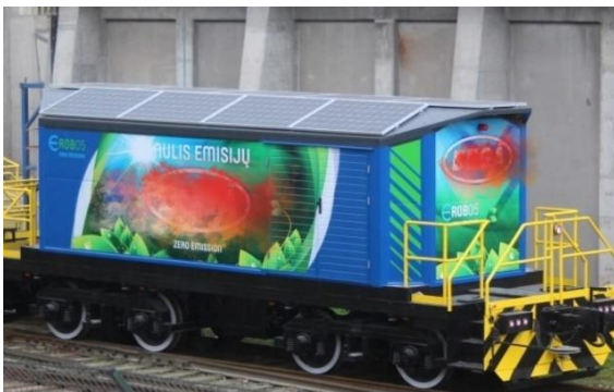
Figure 12. An autonomous robot-locomotive powered by a rechargeable lithium-ion battery
